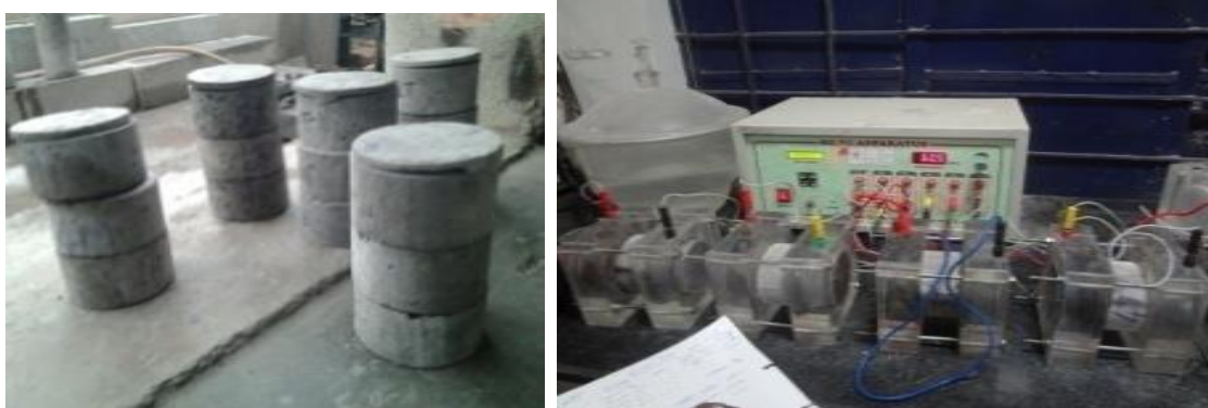
Figure 1: Durability (RCPT) test for 28 days cylinder average test results
