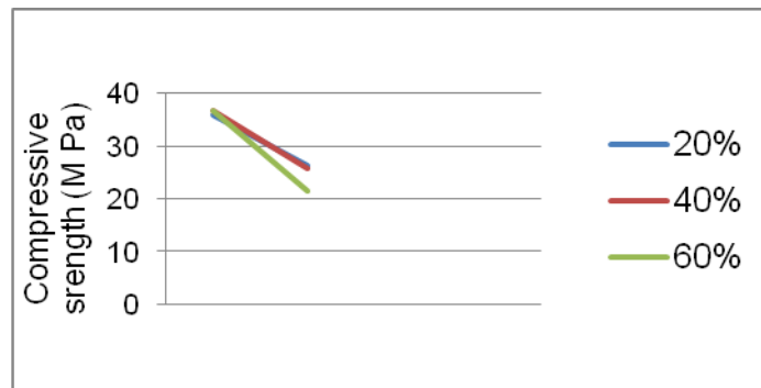
Fig 2: Comparison of compressive strength with different waste stone aggregate
